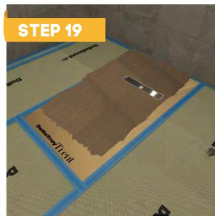
Lay tile adhesive over the tray area and over the gasket up to the drainage aperture ready for the application of tiles.
