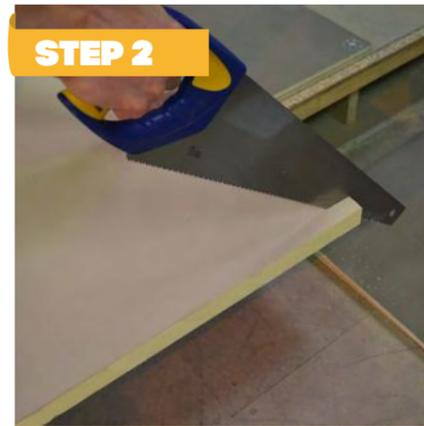
If the drain conflicts with a joist or other obstruction, the tray sides can be trimmed to alter the drain position. Refer to trimming your DeltaTray for details.
